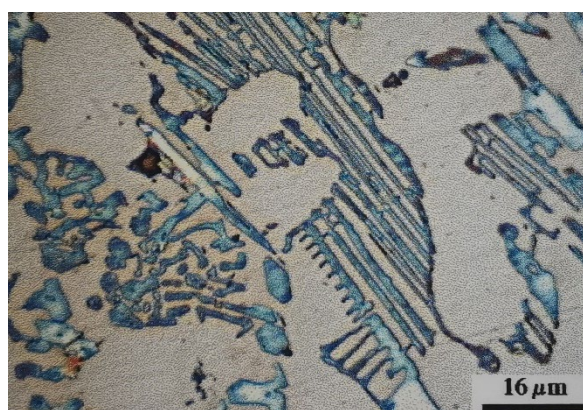
Fig. 2. As-cast microstructure of HCWCI_1, etched in Murakami's reagent
