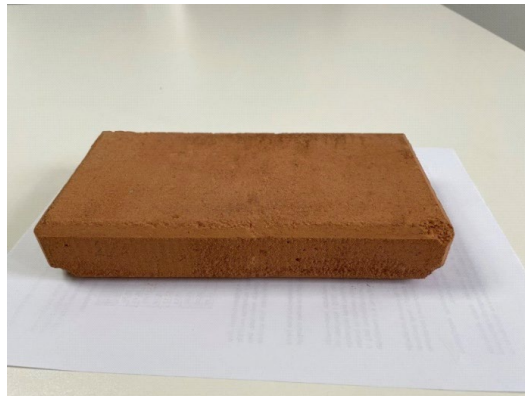
Fig. 1. Brick produced from 100% fly ash using semi-dry pressing technology (Institute for Materials Testing, 2011)
