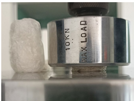
Fig.1. Compression test up to 95% of specimen height
