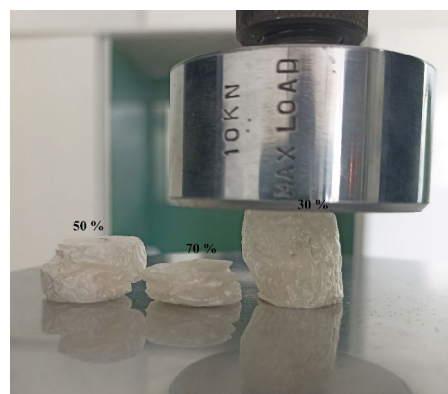
Fig.3. Compression test up to 30 %, 50 % and 70% of specimen height
